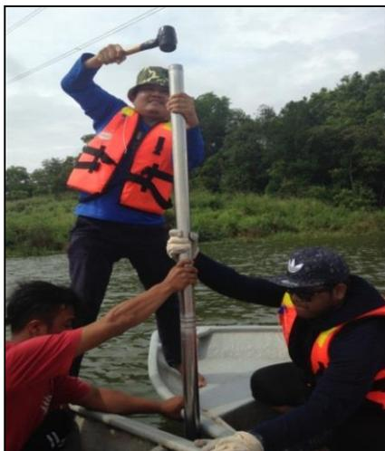
Fig. 2: The gravity corer used to get the sediment
