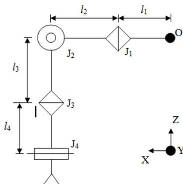
Fig. 1: Structure of robot arm
