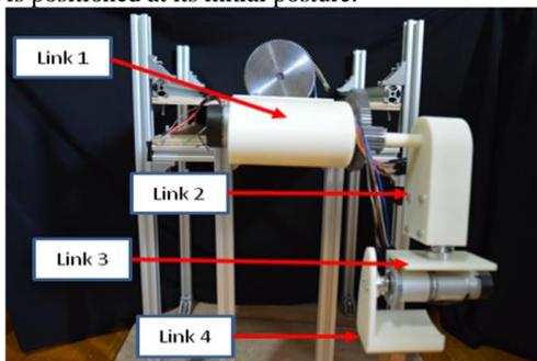
Fig. 5: Assembled robotic arm
