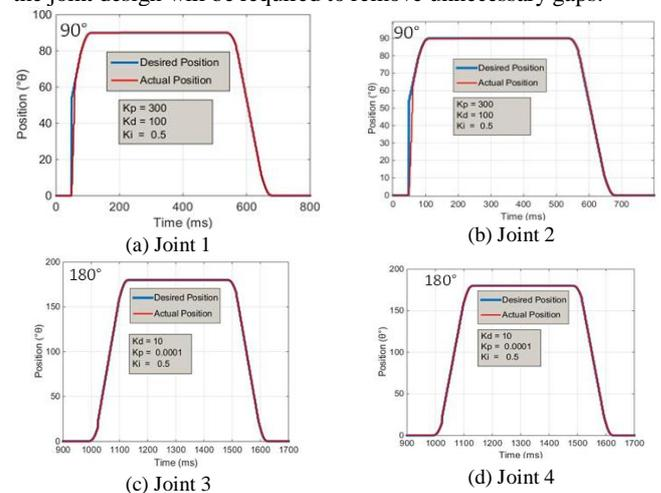
Fig. 7: Transient response of each joint
