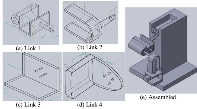
Fig. 3: Robot design on SolidWorks
