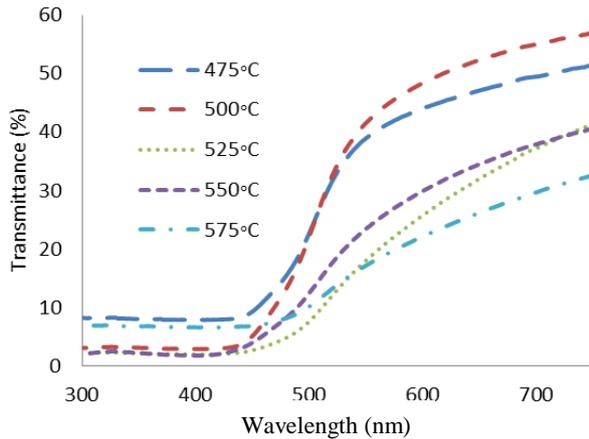
Fig. 7: The transmittance spectra for different annealing temperatures.
