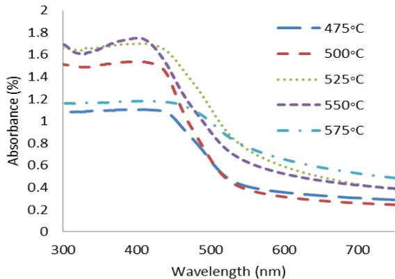
Fig. 8: The absorbance spectra for different annealing temperatures.
