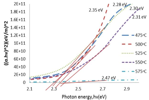
Fig. 10: The optical energy band gap for different annealing temperatures.
