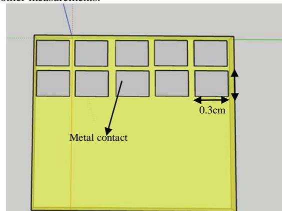
Fig. 3: Top view of the sample with Pt as the metal contact.
