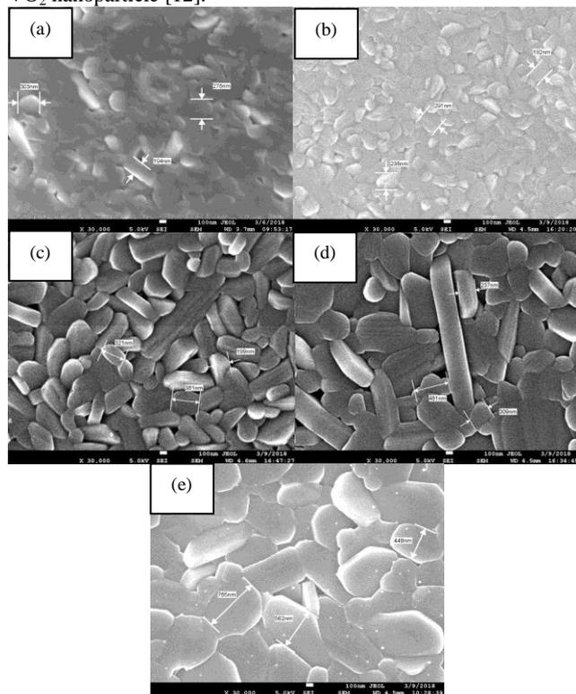
**Fig. 4:** FESEM surface morphology images with different annealing temperature of (a) 475°C, (b) 500°C, (c) 525°C, (d) 550°C and (e) 575°C.
