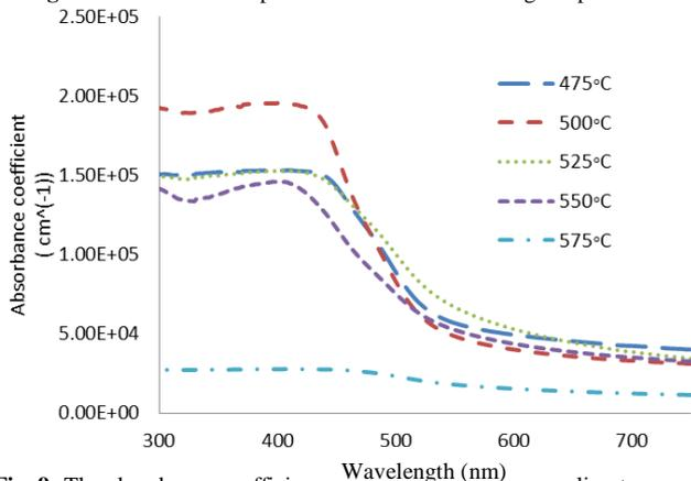
Fig. 9: The absorbance coefficient spectra for different annealing temperatures.
