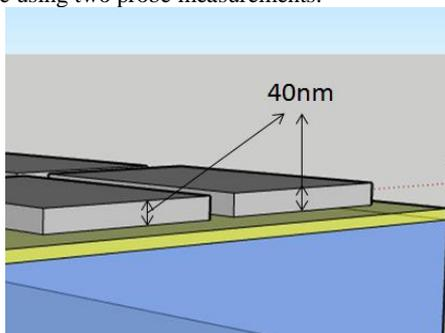
Fig. 1: The side view of sample with Pt metal contact.
