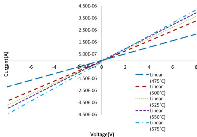
**Fig. 6:** I-V measurement of VO<sub>2</sub> thin films with different annealing temperatures.
