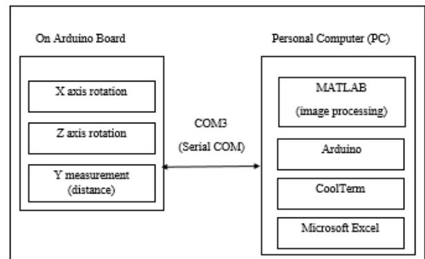
Fig. 2: Block diagram of overall system.
