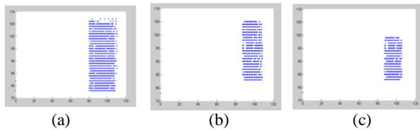
**Fig. 8:** 2D Visualization in MATLAB for the rectangular shape with the distance of (a) 30cm and (b) 40cm (c) 50cm from the infrared sensor.
