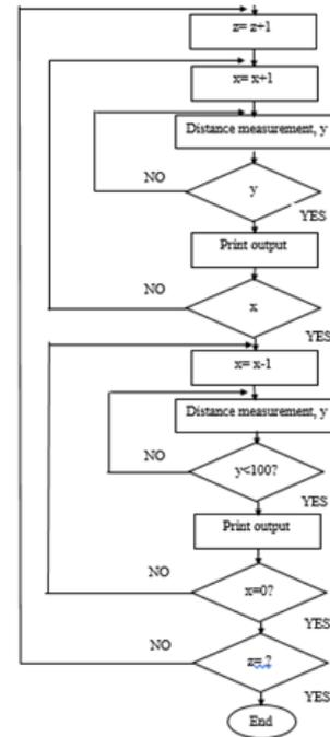
**Fig. 6:** Control algorithm flow in the Arduino hardware platform.
