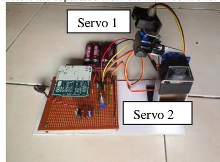
Fig. 4: Hardware design of the rotating infrared sensor for multiple scanning operations.
