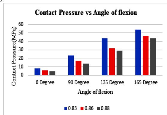
**Fig. 6:** Contact pressure (MPa) versus angle of flexion for 0.83, 0.86 and 0.88 conformity values
