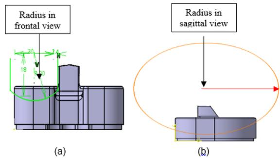
**Fig. 5:** (a) Radius of Tibial in frontal view (RTF) and (b) Radius of Tibial in sagittal view (RTS)
