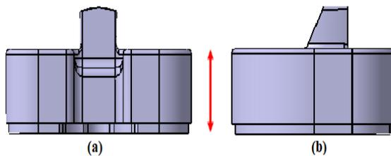
**Fig. 4:** The minimum thickness of tibial insert labeled with a red double arrow in (a) anterior view and (b) lateral view of UHMWPE tibial insert.
