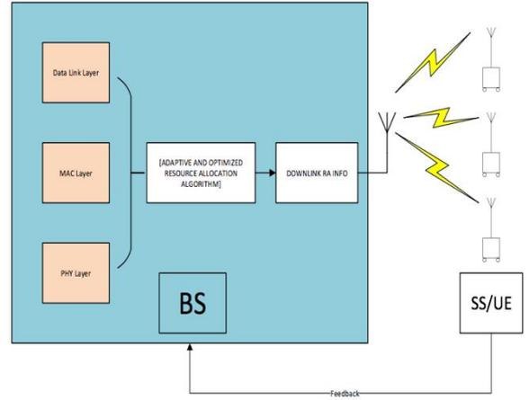
Fig. 3: Cross Layer Solution model for OFDMA based resource allocation in connection oriented networks.
