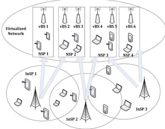
Fig. 2: Conceptual framework for Wireless Network Virtualization [2].
