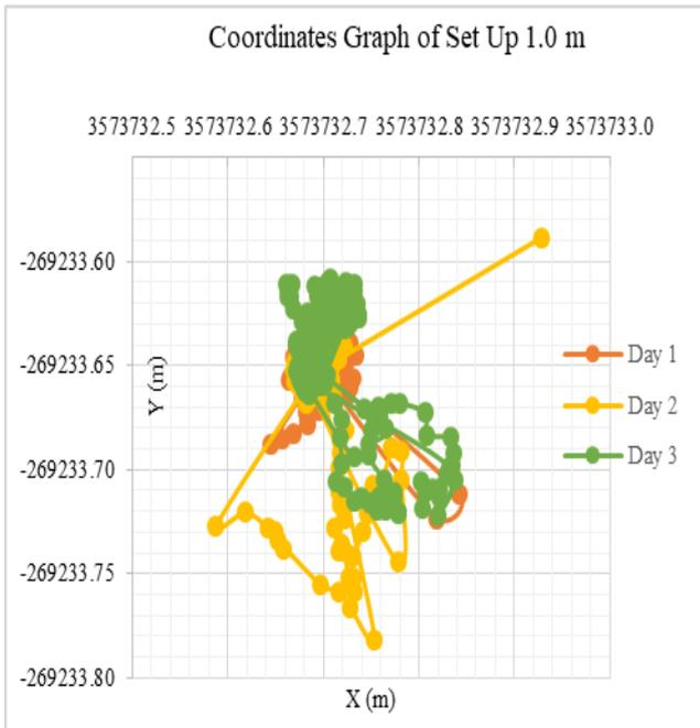
Fig. 1: Coordinates of X-ECEF and Y-ECEF for Set Up 1.0 m (x-axis and y-axis represent coordinate)
