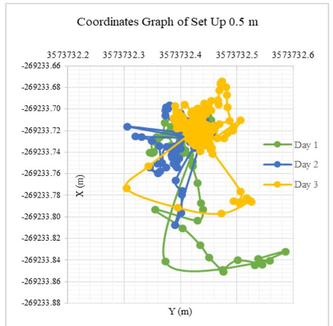
Fig. 4: Coordinates of X-ECEF and Y-ECEF for Set Up 0.5 m (x-axis and y-axis represent coordinate)
