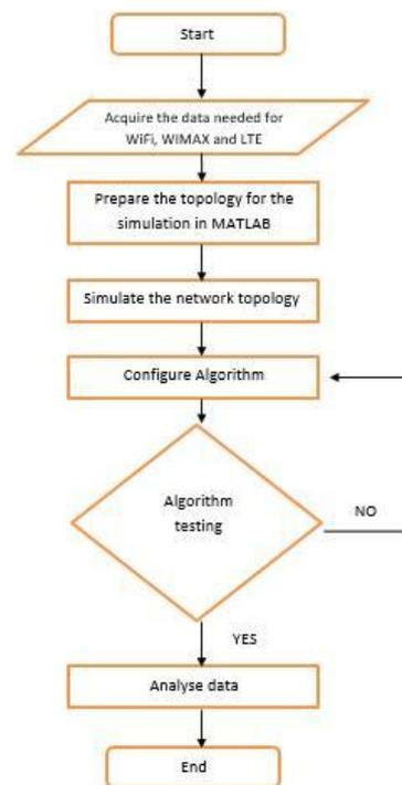
Fig. 2:. Simulation Process Diagram
