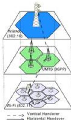
Fig. 1. Differences between Vertical and Horizontal Handover
