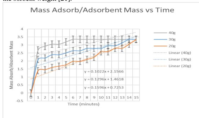
**Fig. 5:** Mass Adsorb/Adsorbent Mass vs Time of Biochar
