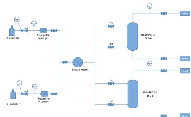
Fig. 1: Adsorption Unit Schematic Diagram
