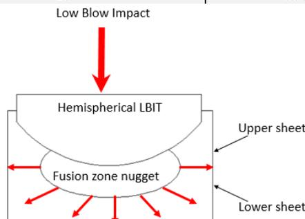
Fig. 2: Schematic illustration of LBIT process
