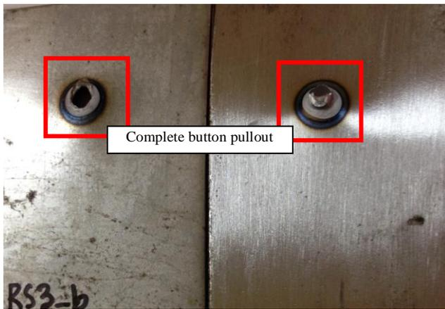
Fig. 4: Failure mode of 20 Joule LBIT samples.
