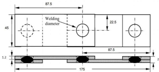
Fig. 1: Spot welding sample dimension
