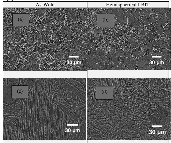
Fig. 3: Microstructure changes of (a) HAZ as-welded, (b) HAZ 20 Joule LBIT (c) fusion zone as-welded and (d) fusion zone 20 Joule LBIT
