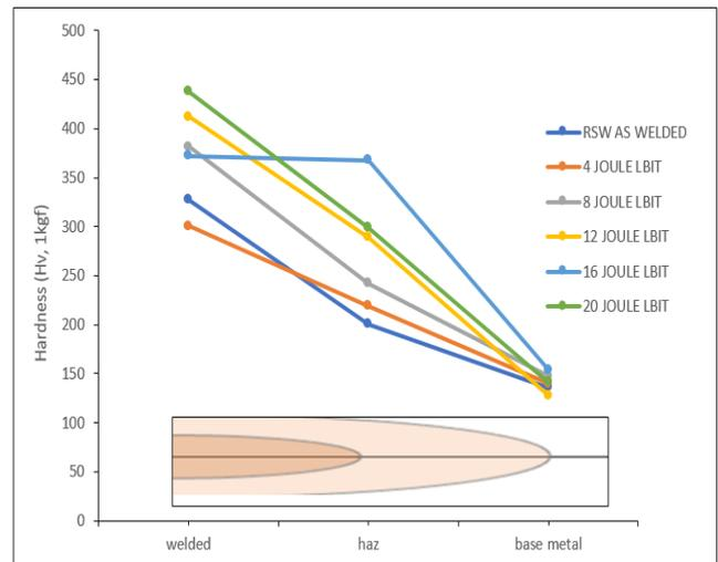
Fig. 6: Hardness profile of the samples.
