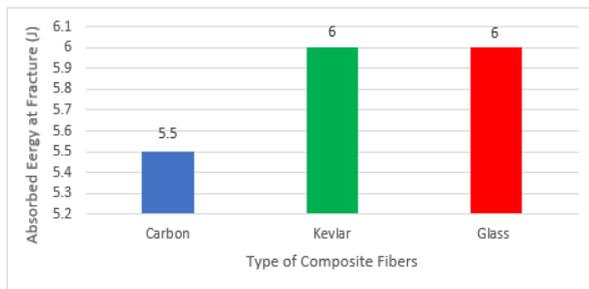
**Fig. 7:** Impact energy of each composite specimens
