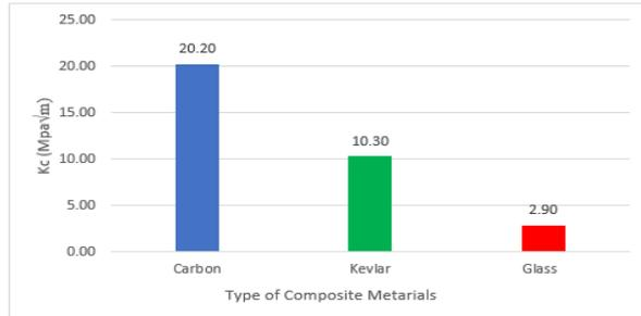
**Fig. 6:** Fracture toughness of each composite specimens
