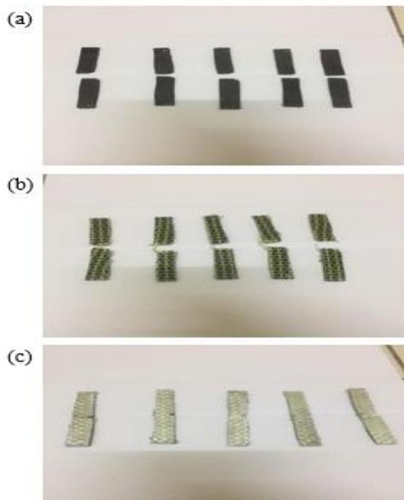
**Fig. 8:** Sample of three composite specimens after impact test; (a) woven carbon fiber, (b) woven Kevlar and (c) woven glass fiber
