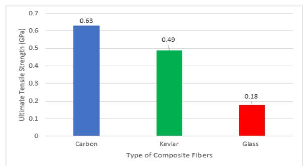
Fig. 4: Ultimate Tensile Strength of each composite specimens.
