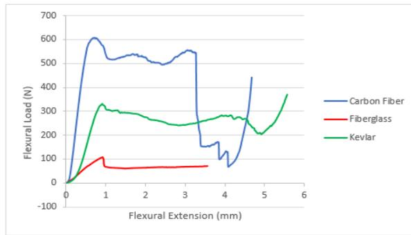
**Fig. 5:** Experimental flexural load-displacement curve for three types of composite specimens
