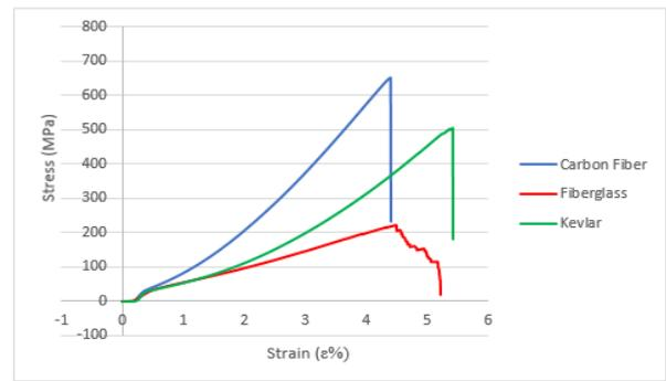
Fig. 2: Experimental tensile stress-strain curve for three types of composite specimens
