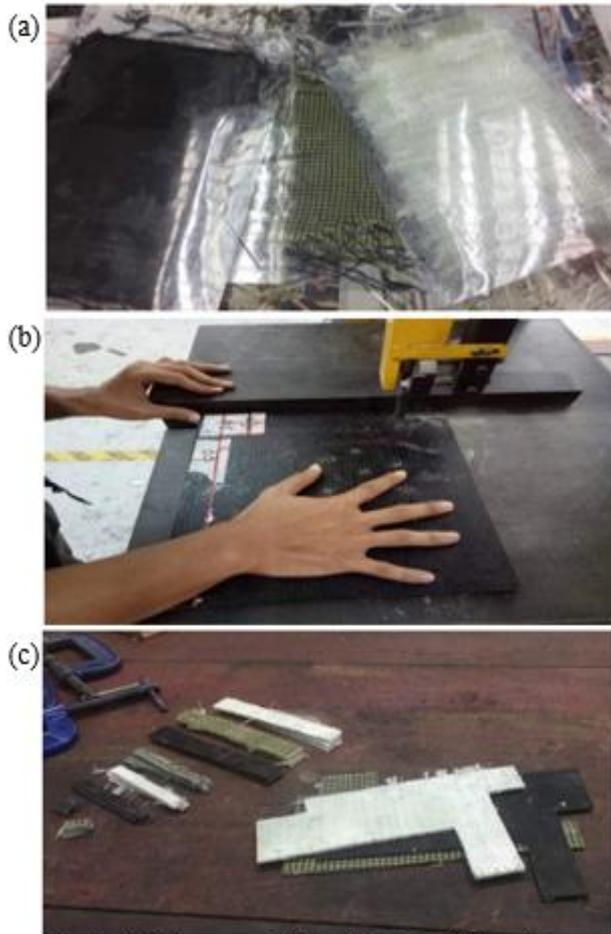
Fig. 1: (a) Woven-type Carbon, Kevlar and Glass fibers were used as specimens; (b) cutting specimens by vertical band saw; (c) small specimens for different mechanical tests.
