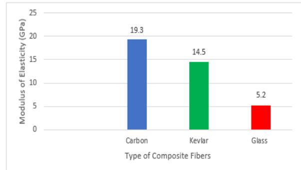
Fig. 3: Modulus of Elasticity of each composite specimens
