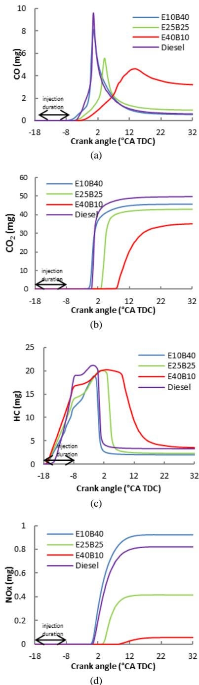
**Fig. 4:** CO (a), CO<sub>2</sub> (b), HC (c) and NO<sub>x</sub> (d) emission of diesel-ethanol-PME blends at 1600 RPM engine speed
