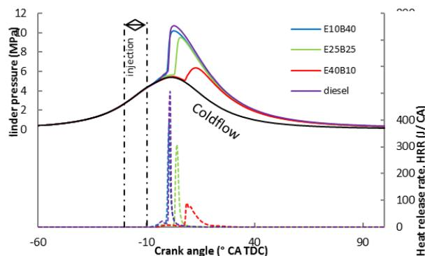
**Fig. 2:** In-cylinder pressure and heat release rate (HRR) profile of diesel-ethanol-PME blends at 1600 RPM engine speed.
