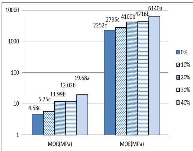
Fig. 1: Effect of strands ratio on the MOR and MOE of rice husk particleboard
