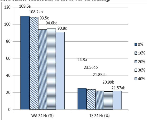
Fig. 2: Effect of strands ratio on the TS and WA of rice husk particleboard
