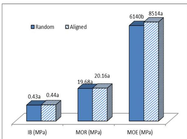
Fig. 3: Effect of *A. excelsa* strands arrangement on the mechanical properties of rice husk particleboard
