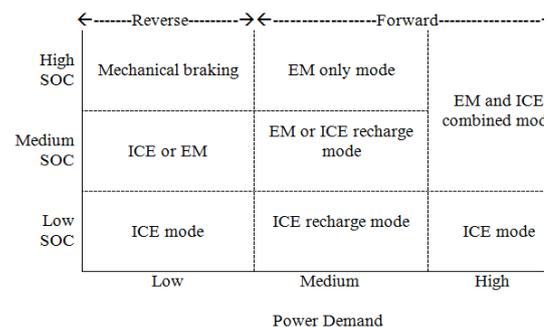
Fig 5: PHERB EMS modes of operation.
