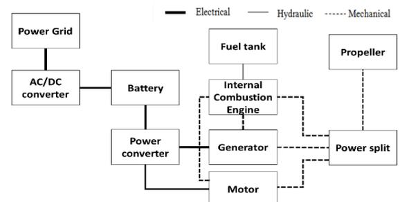
Fig. 2: Block diagram of the PHEB powertrain
