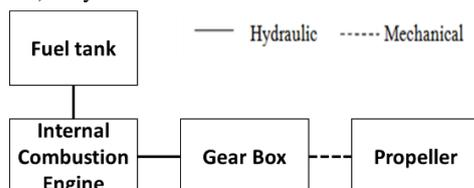
Fig. 1: Block diagram of the CB powertrain
