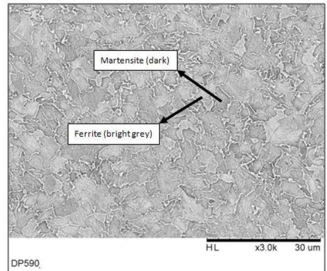
**Fig. 2:** Microstructure DP590 using Scanning Electron Microscope.
