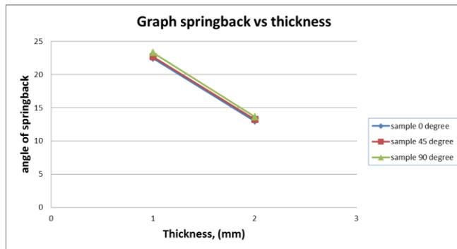
Fig. 4: Springback angle vs thickness
