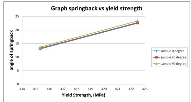
Fig. 5: Springback angle vs yield strength
