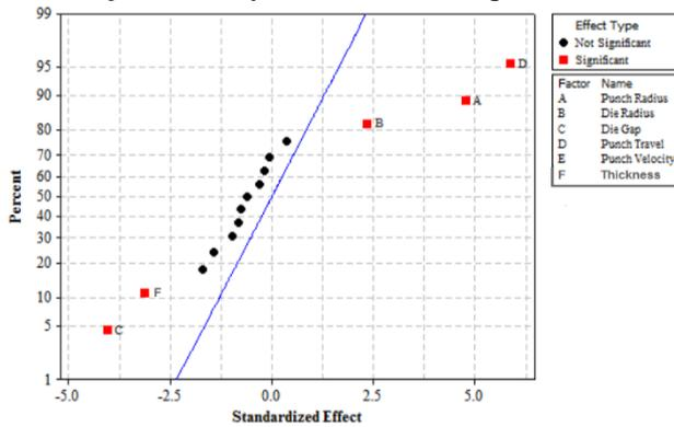
Fig. 7: Parameters that affecting springback for experiment
