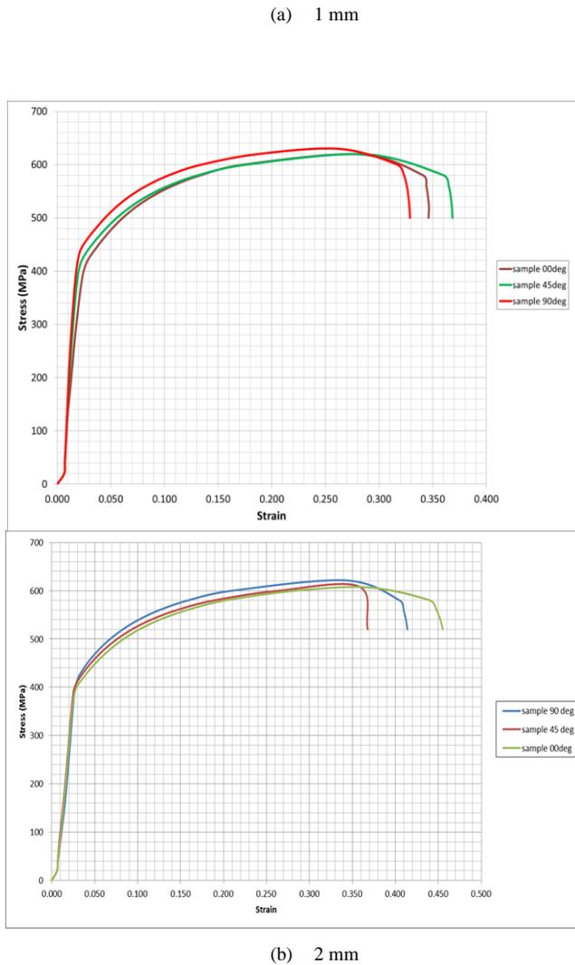
Fig. 3: Stress vs strain curve of DP590 at various thicknesses; (a) 1 mm and (b) 2 mm in different direction
