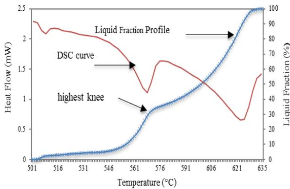
**Fig 2:** DSC heating flow and liquid fraction curves of Al-5.7Si-2Cu-0.3Mg Alloy.
