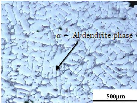
**Fig.1:** Microstructures of as received Al-5.7Si-2Cu-0.3Mg Alloy with dendritic structure
