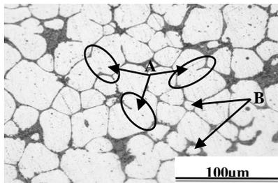
**Fig 8:** Close-up microstructure of Al-5.7Si-2Cu-0.3Mg alloys after reheating trial at 600 °C.
