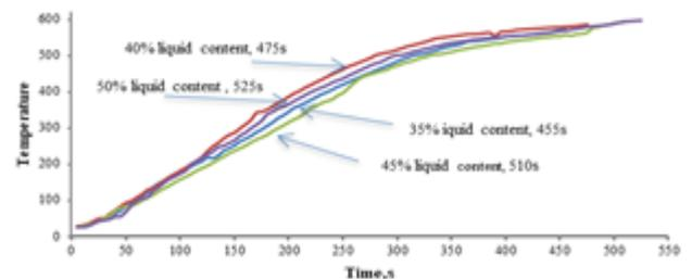
**Fig 7:** Reheating trial at different liquid content.
