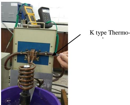
**Fig 3:** Experimental setup for reheating process via coil induction during the reheating process.
