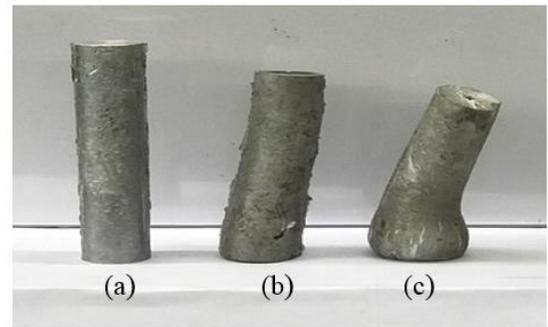
**Fig 10:** Billet of Al-5.7Si-2Cu-0.3Mg alloy (a) Initial condition before reheating,  $t = 0\text{s}$  (b) 45% liquid contents at 595 °C,  $t = 510\text{s}$  (c) 50% liquid content at 600 °C,  $t = 535\text{s}$ .
