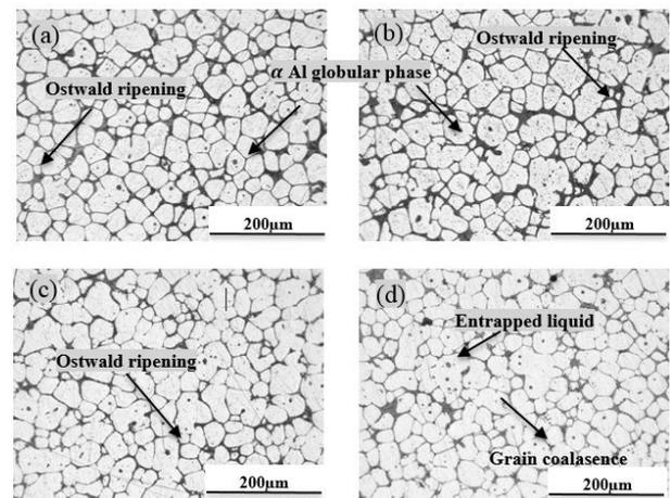
**Fig 5:** Microstructure of Al-5.7Si-2Cu-0.3Mg Alloy quenched after reheating. (a) at 35% liquid content (b) at 40% liquid content. (c) at 45% liquid content (d) at 50% liquid content.
