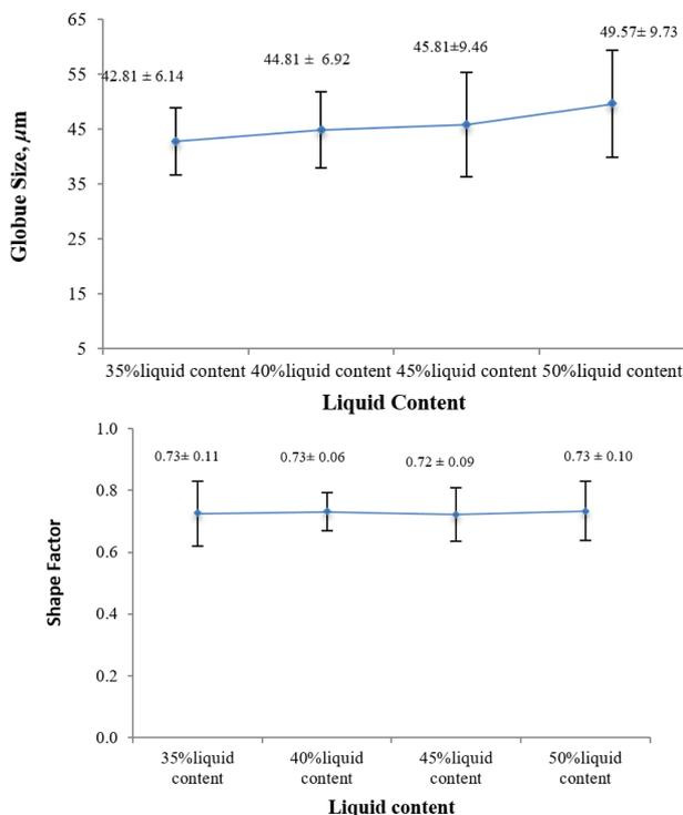
**Fig 9:** Globule size and shape factor of Al-5.7Si-2Cu-0.3Mg alloys at different liquid content.
