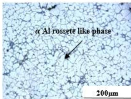
**Fig 4:** Microstructures of as cooling slope casting of Al-5.7Si-2Cu-0.3Mg alloy at 650°C with a cooling slope length of 400m.
