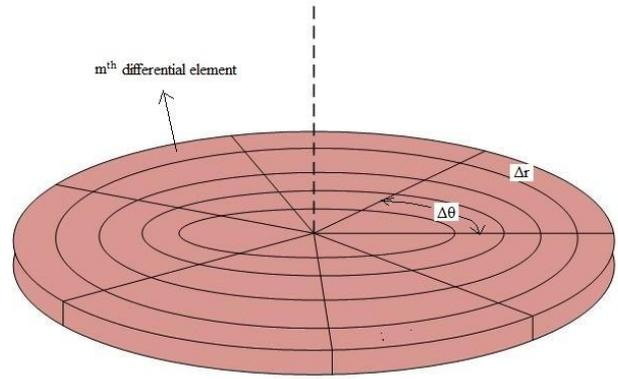
Fig. 2: Disc discretization into 'm' differential elements
