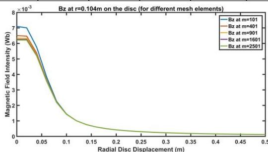
**Fig. 13:** Magnetic Field at r=0.104m radius of the non-coaxial disc
