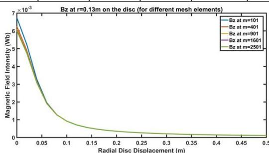
**Fig. 14:** Magnetic Field at r=0.13m radius of the non-coaxial disc
