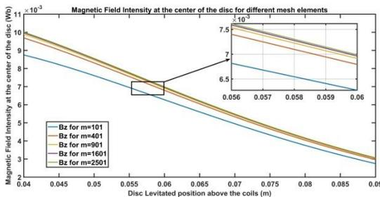
**Fig. 3:** Magnetic Field at the centre of the disc
