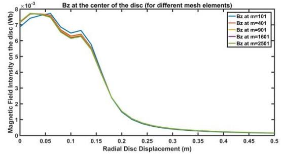
**Fig. 9:** Magnetic Field at  $r=0m$  radius of the non-coaxial disc
