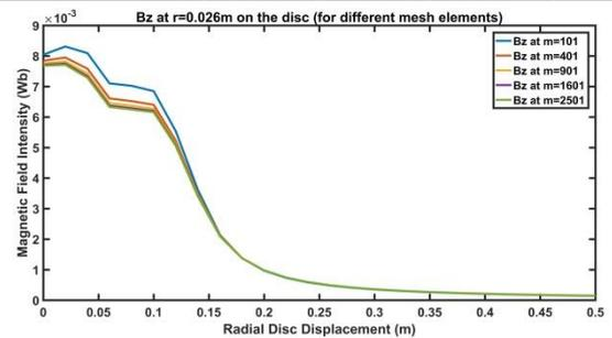
**Fig. 10:** Magnetic Field at  $r=0.026m$  radius of the non-coaxial disc
