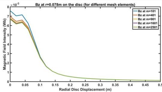
**Fig. 12:** Magnetic Field at r=0.078m radius of the non-coaxial disc
