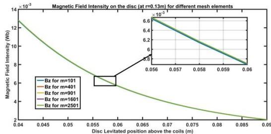
**Fig. 8:** Magnetic Field at  $r=0.13m$  radius of the disc
