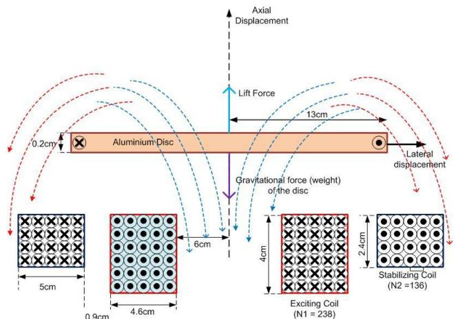
Fig. 1: Principle of Magnetic Levitation due to repulsive force.
