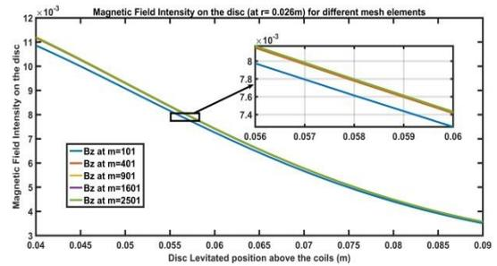
**Fig. 4:** Magnetic Field at  $r=0.026m$  radius of the disc
