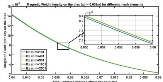
**Fig. 5:** Magnetic Field at  $r=0.052m$  radius of the disc
