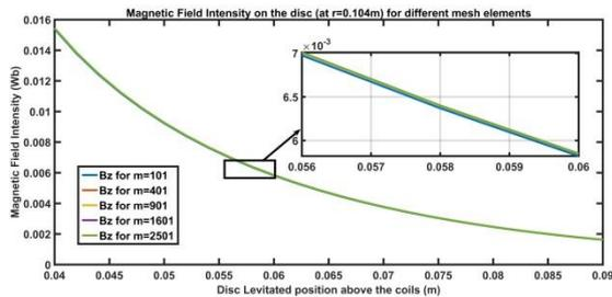
**Fig. 7:** Magnetic Field at  $r=0.104m$  radius of the disc
