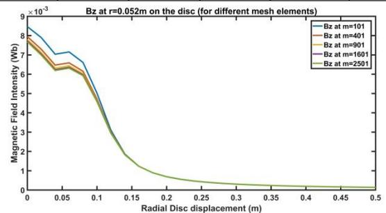
**Fig. 11:** Magnetic Field at  $r=0.052m$  radius of the non-coaxial disc
