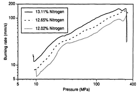
Fig. 3: Burn Rate Curves for Grains with Zero Perforations and Various Nitrogen Levels [13]
