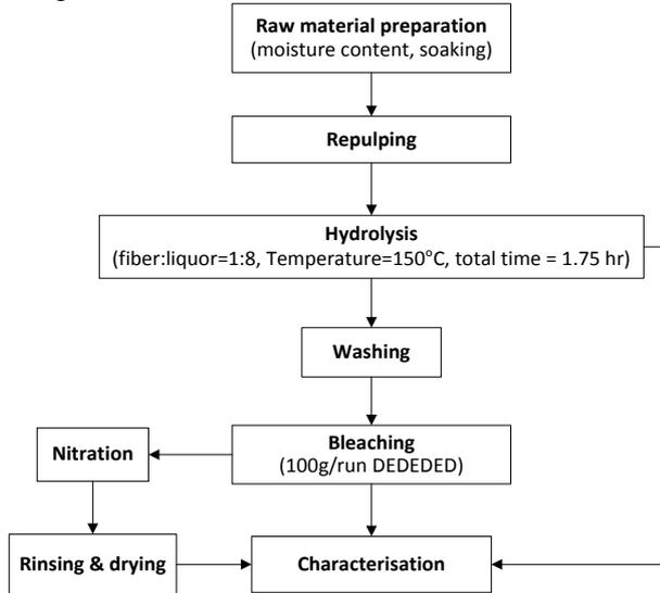
Fig.9: Overall nitrocellulose process flow for EFB
