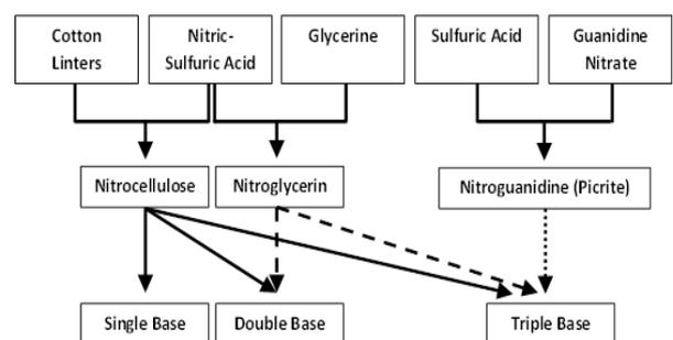
Fig. 5: Nitrocellulose Based Propellants
