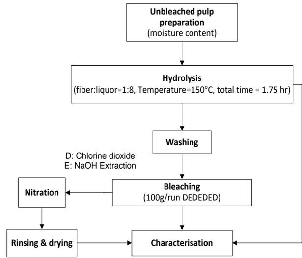
Fig.11: Overall nitrocellulose process flow for Kenaf Bast
