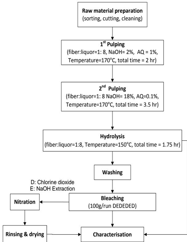
Fig.10: Overall nitrocellulose process flow for Rhizophora
