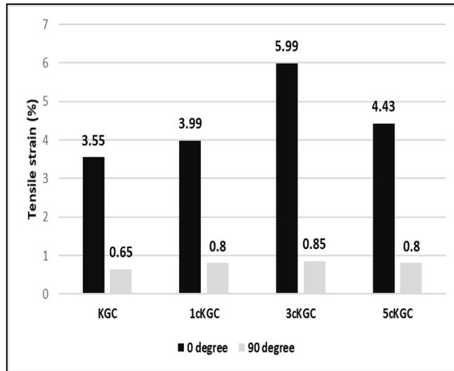
Figure 6: Tensile strain of kenaf glass fibre composite
