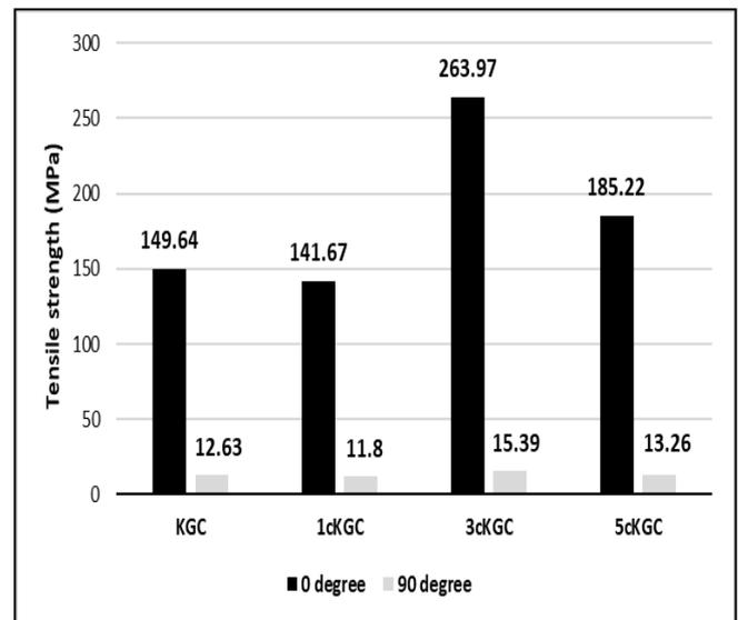
**Figure 5:** Tensile strength of kenaf glass fibre composite
