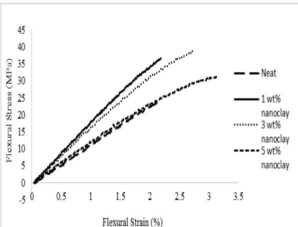
Fig.4: Flexural stress-strain curves of nanoclay filled BFRP composites compared to neat BFRP
