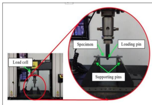
**Fig. 2:** Three-point bending flexural test setup using Instron 3382 Universal Testing Machine
