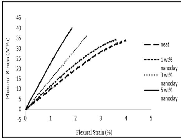
Fig. 3: Flexural stress-strain curves of nanoclay modified epoxy polymer compared to neat polymer
