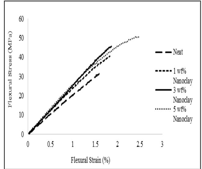
Fig. 5: Flexural stress-strain of curves nanoclay filled GFRP composites compared to neat GFRP
