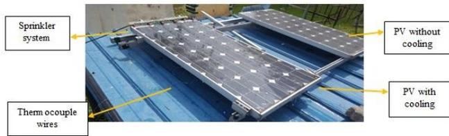
Fig. 3: Experiment setup at GER, UiTM Shah Alam
