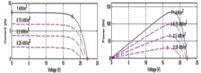
Fig. 3: Power vs Voltage & Current vs Voltage graphs from PV panel model.
