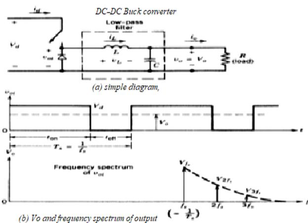
Fig.5: DC-DC Buck converter (a) simple diagram, (b)  $V_o$  and frequency spectrum of output
