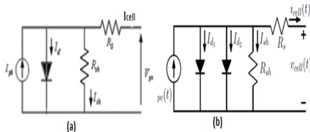
Fig. 2: (a) PV cell Equivalent circuit (b) PV panel, double-diode model.
