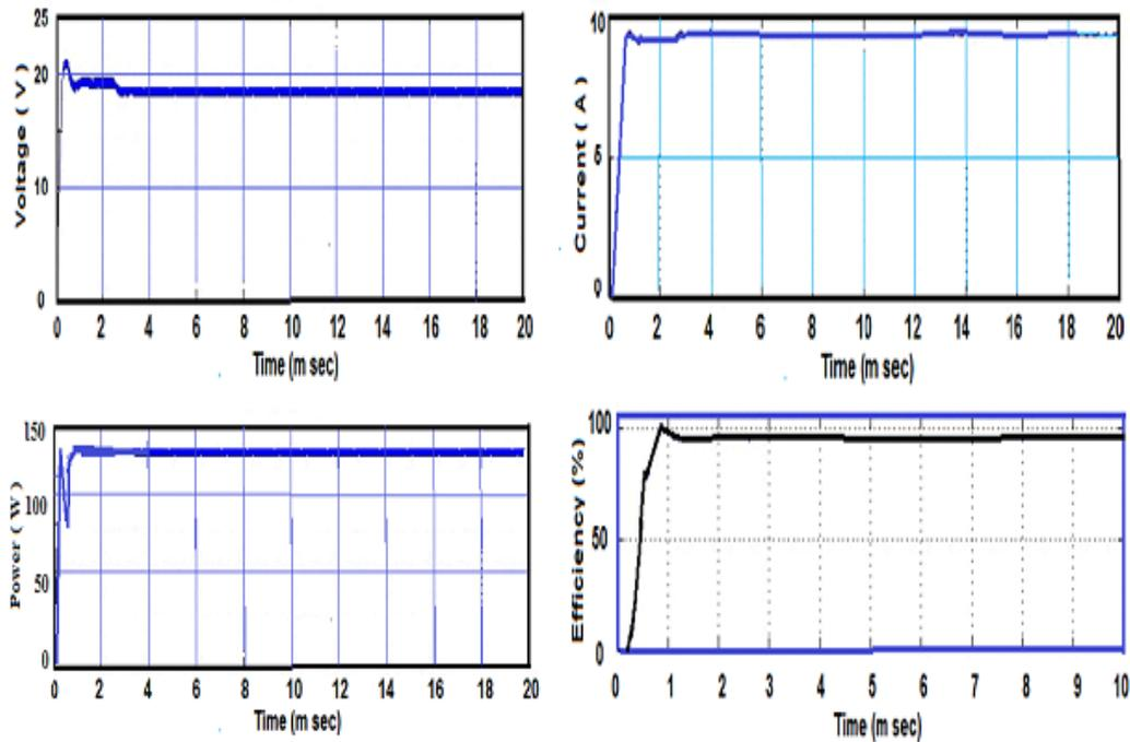
Fig. 7: Efficiency and output voltage, current, and power at constant irradiation.
