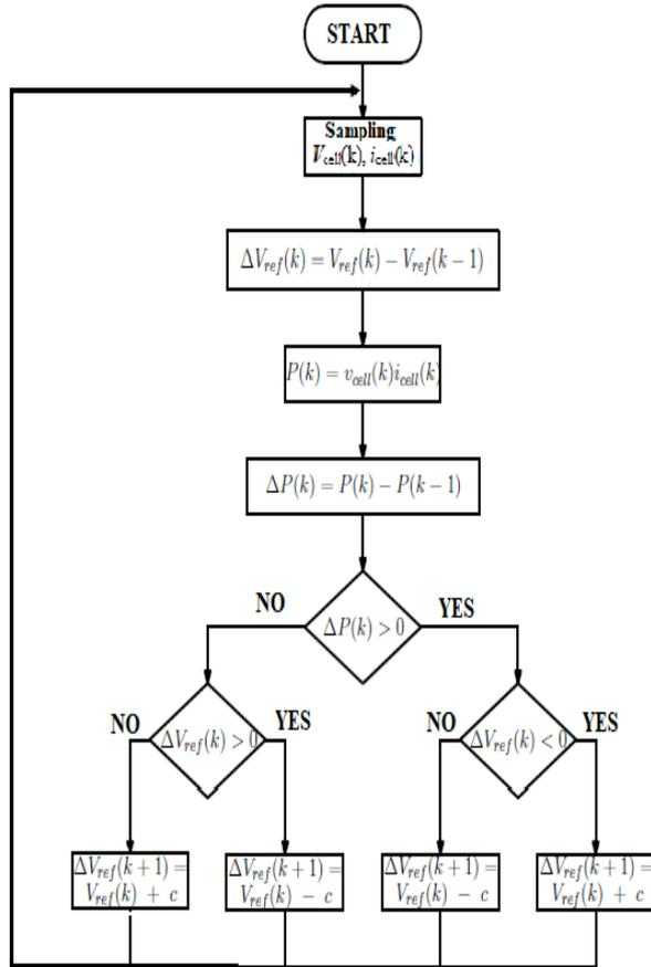
Fig. 3: flow chart of P&O algorithm
