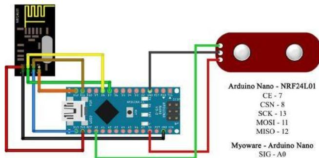
**Figure 3.1** Schematic Diagram for Electromyogram Sensor
