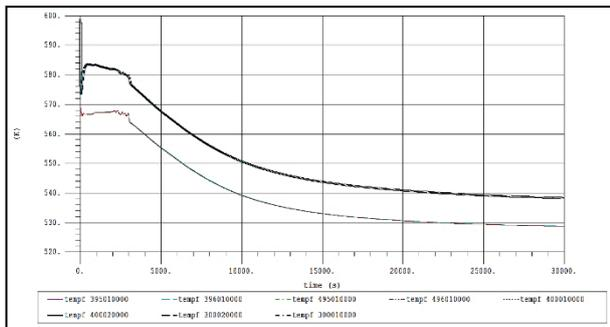
Fig. 8: Outlet and Inlet Temperatures of the Reactor Pressure Vessel.
