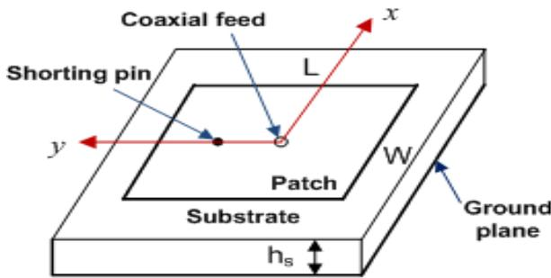
Fig. 3: Shorting Pin Loaded Configuration.
