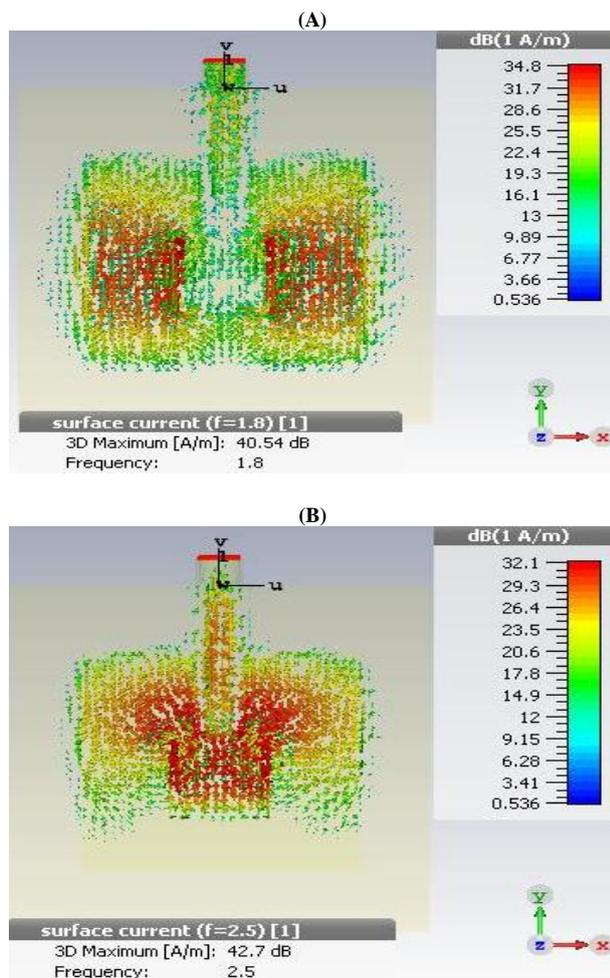
Fig. 7: Simulated Current Distribution at A) 1.8 GHz and B) 2.5 GHz.
