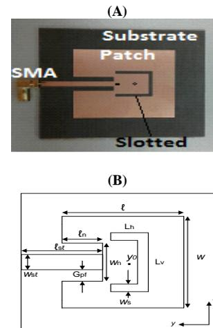
**Fig. 2:** The A) Fabricated and B) Geometry Layout of the Proposed Design.
