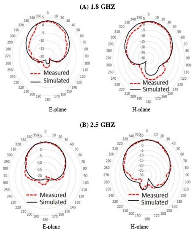
Fig. 6: Radiation Patterns of Realized Gain at (A) 1.8 GHz and (B) 2.5 GHz.
