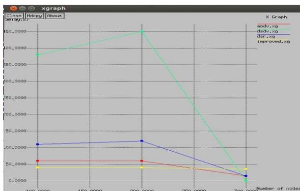
Fig. 6: End-to-End Delay Comparison.
