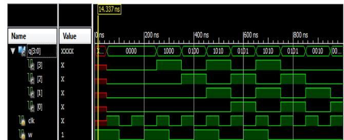
Fig.19: Simulation output of Proposed Shift right Register using Reversible Logic
