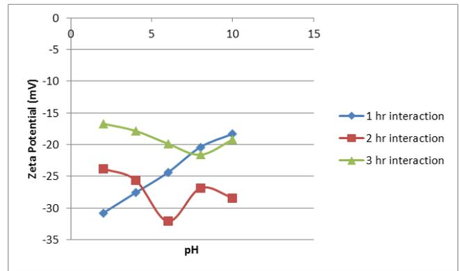
Potential of ore with bacterial interaction at different pH
