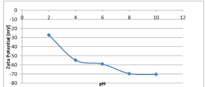
Potential of ore without bacterial interaction at different pH Further, in order to study the microbe mineral interactions studies were carried out on the copper ore .
