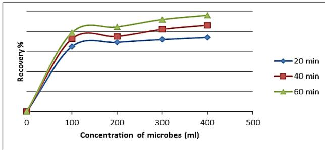
Increase in Copper % in copper concentrate with increase in interaction time
