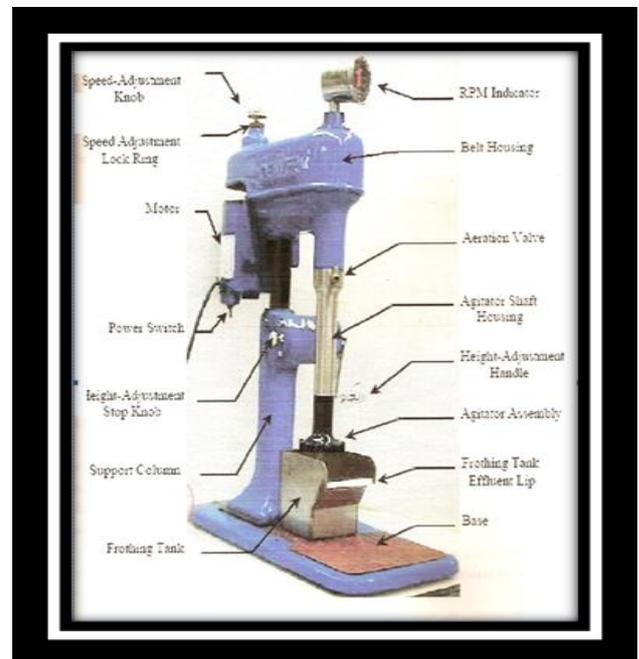
Fig.3: Denver Flotation Cell
