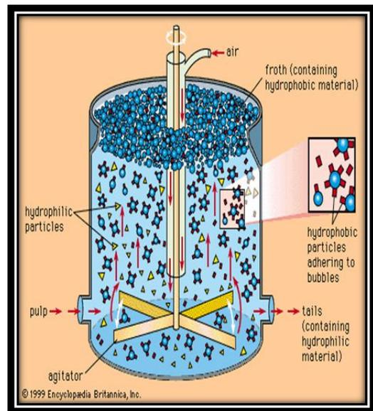
Fig.2: Flotation Mechanism
