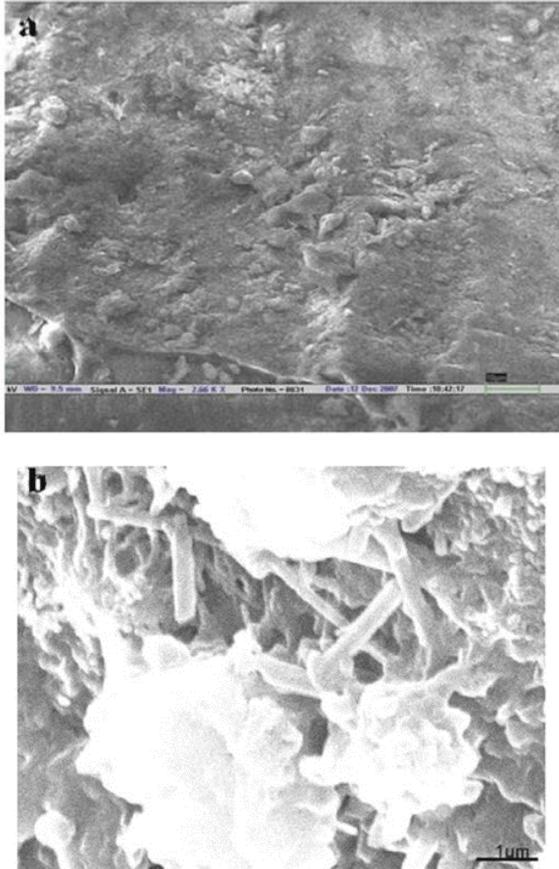
**Fig. 4:** SEM showing bacterial calcite precipitation in cracks of concrete: (a) sample of cement mortar without bacteria, (b) sample taken nearby to surface of healed crack, displaying calcite crystals with rod formed *Bacillus* sp. CT-5.
