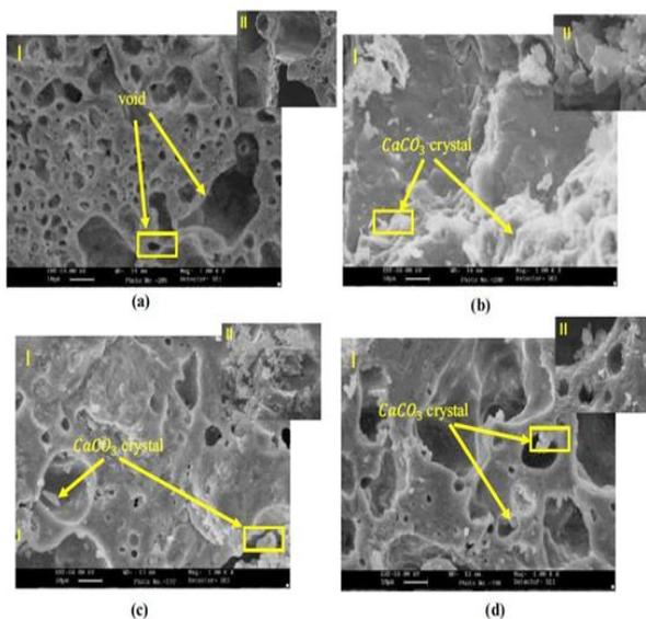
**Fig. 5:** SEM of (a) Specimens without bacteria submerged in water; (b) Specimens with bacteria in aggregates and mixing water; (c) Specimens with bacteria in mixing water; (d) Specimens cast with aggregates filled with bacteria sediment submerged in Urea-CaCl<sub>2</sub>.
