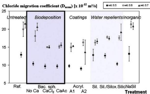
Fig. 3: Chloride migration coefficients,  $D_{nssm}$ , for distinctive grades of applied with different kinds of surface treatments.
