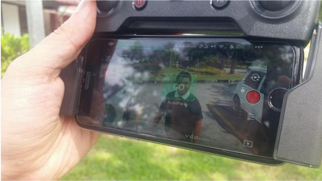
**Fig. 4:** A mobile phone connected to the drone remote for viewing and monitoring of the video shots captured by the drone
