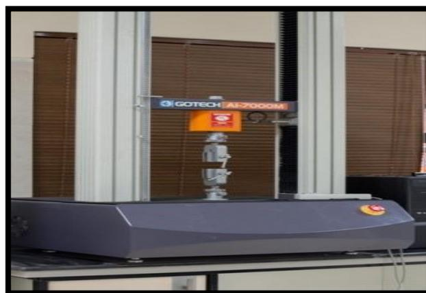
Fig. 1: GOTECH AI-7000M Tensile Testing Machine Used in This Research.
