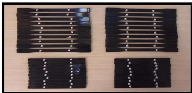
Fig. 3: The Produced Nanocomposite Samples Containing [1] wt. % Carbon Nanotube and 99 wt. % Polyethylene.
