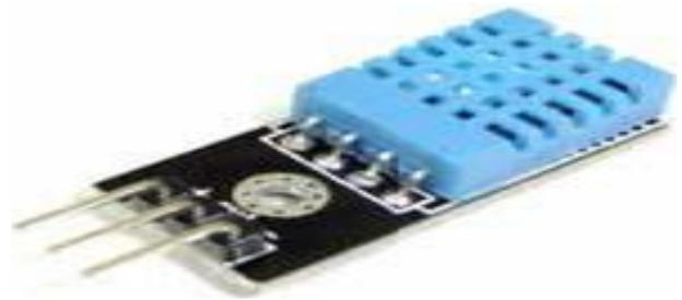
Fig. 2: DHT11 Temperature and Humidity Sensor.
