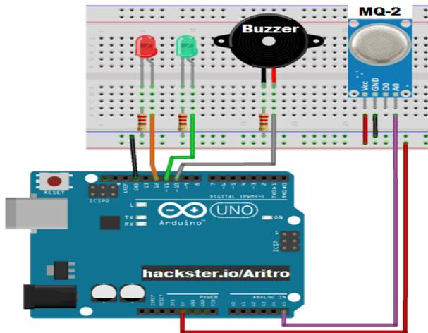
Fig. 6: MQ2 - Smoke Sensor.
