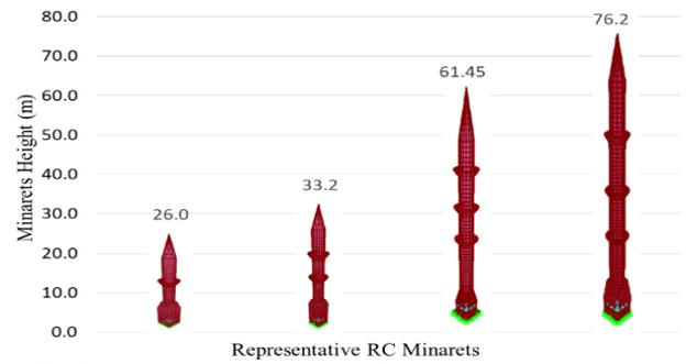
Fig. 7: 3-D Finite Element Models of the Representative Minarets.
