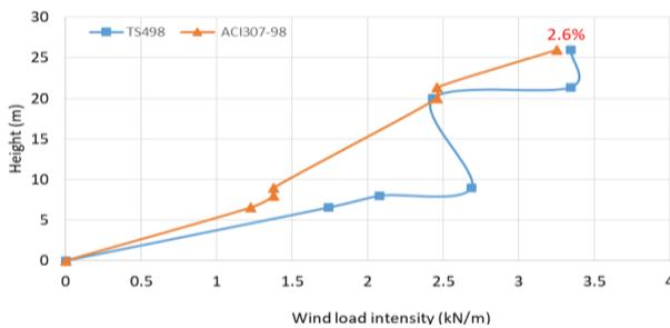
**Fig. 10:** Comparison of Wind Load Intensities for 26.0 M Minaret.
