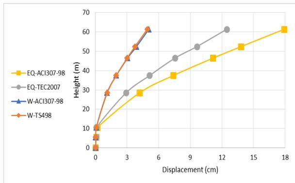
Fig. 18: Displacements over the Height of 61.45 M Minaret.
