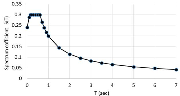
**Fig. 14:** Design Response Spectrum Curve According to TEC2007.
