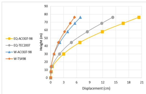
Fig. 19: Displacements over the Height of 76.2 M Minaret.
