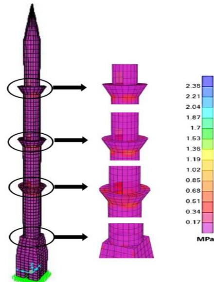
Fig. 21: Normal and Shear Stress Distribution of 76.2 M Minaret.
