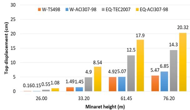
Fig. 20: Top Displacements Due To Wind and Earthquake Loads.
