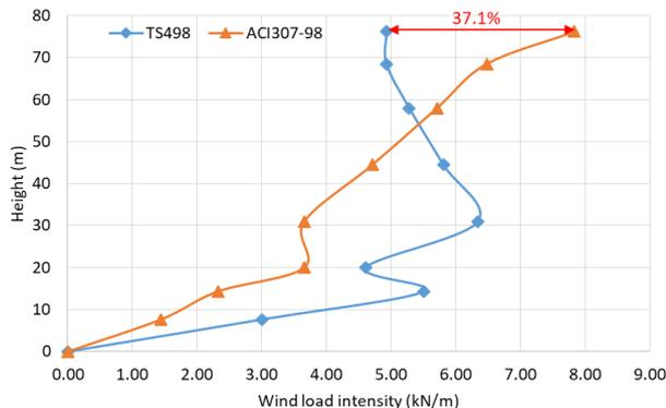
**Fig. 13:** Comparison of Wind Load Intensities for 76.2 M Minaret.
