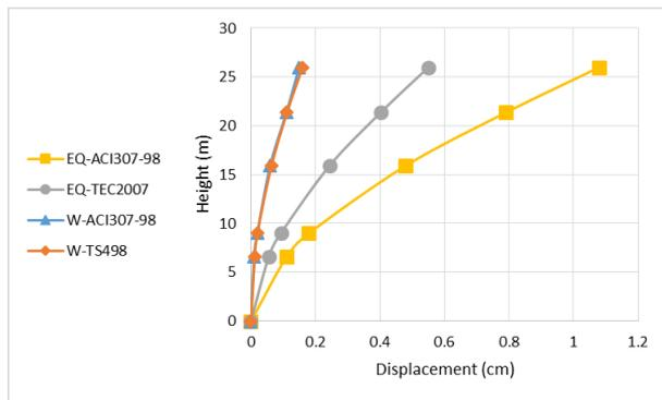
Fig. 16: Displacements over the Height of 26.0 M Minaret.
