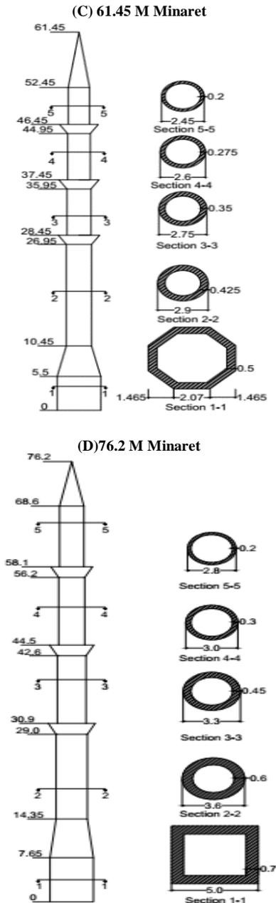
Fig. 6: Geometrical and Cross Sectional Properties of the Selected Minarets (Dimensions Are in Meters and Drawings are Not to Scale).
