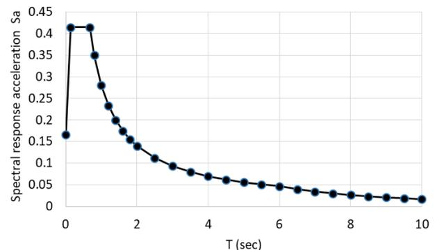
**Fig. 15:** Design Response Spectrum Curve According to ACI307-98.
