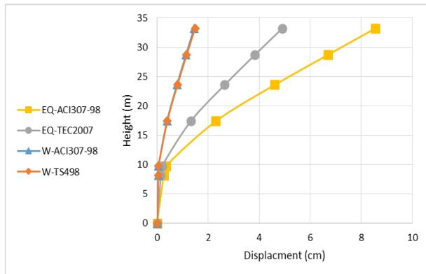
Fig. 17: Displacements over the Height of 33.2 M Minaret.
