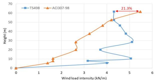
**Fig. 12:** Comparison of Wind Load Intensities for 61.45 M Minaret.
