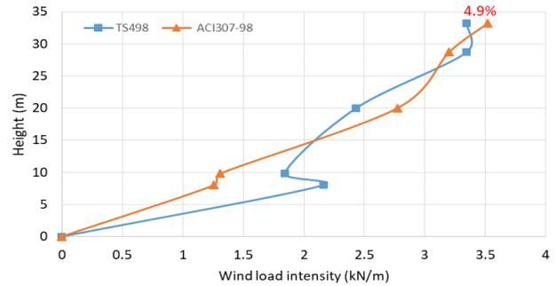
**Fig. 11:** Comparison of Wind Load Intensities for 33.2 M Minaret.
