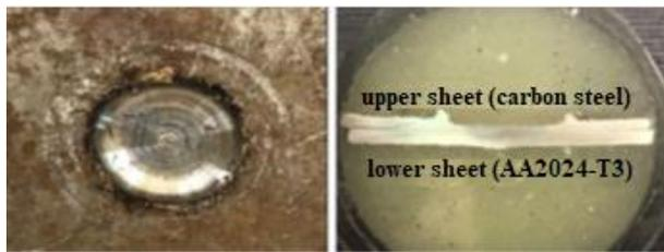
Fig. 9: Macrostructure Photographs of Cross-Section of Dissimilar FSSW Joints.
