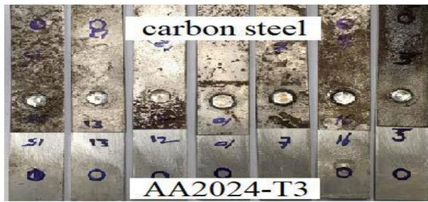
Fig.8: Samples of Welded Specimens.
