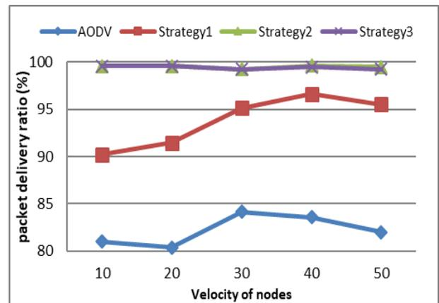
Fig. 5:PDR versus Vehicle's Velocity.
