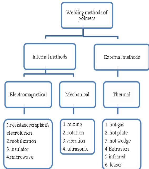
Fig. 2: Welding methods for thermoplastics [16]
