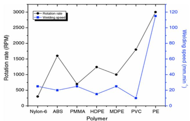
Fig. 3: Some FSW parameters for different polymers [19]
