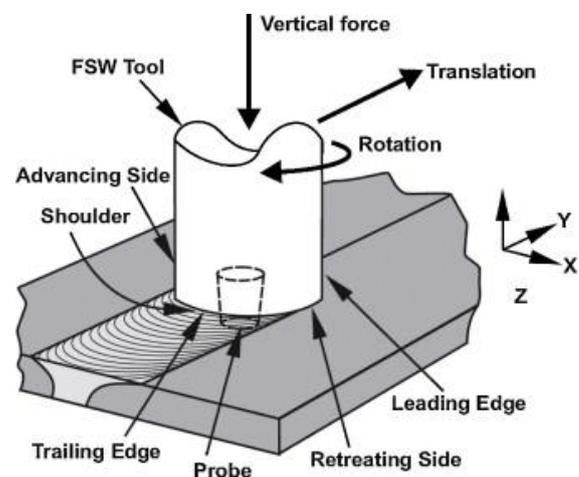
Fig. 1: The schematic of FSW method [3]
