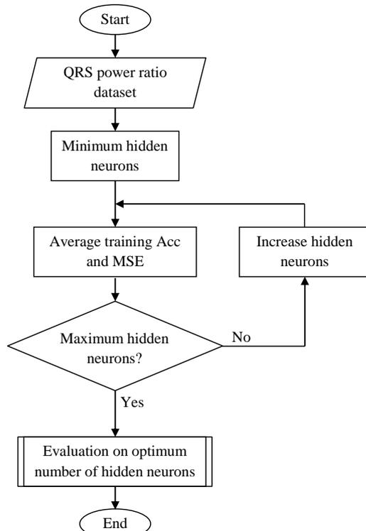
Fig. 2: Exhaustive search algorithm. MSE = Mean Squared Error.
