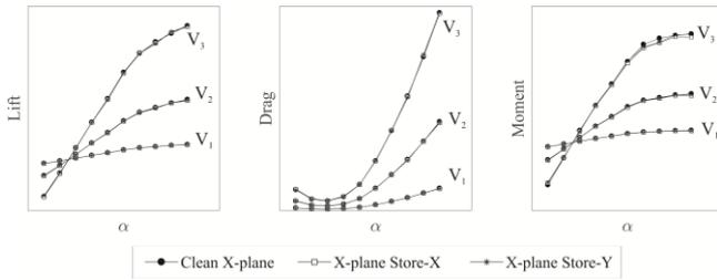
Fig. 5: Lift, drag and moment forces
