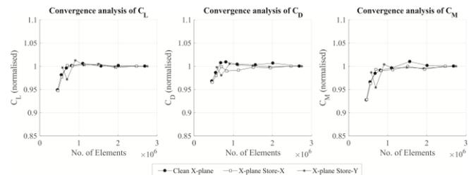
**Fig. 4: Convergence analysis of aerodynamic coefficients at  $\alpha = 15^\circ$**
