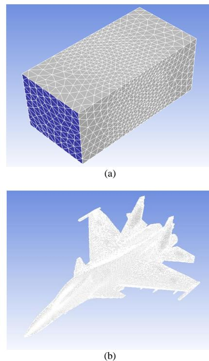
**Fig. 3: Computational domain and X-plane model ready for calculation**
