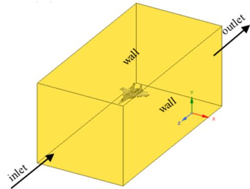
**Fig. 2: X-plane model inside the computational domain**
