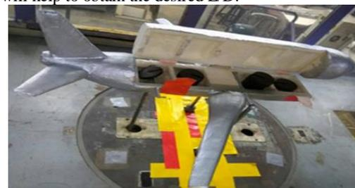
**Fig. 8:** Weights inside the aircraft model
