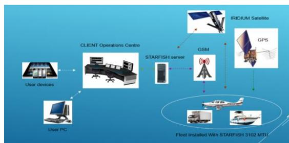
Fig. 2: System architecture (Courtesy of Worldgate Technologies)
