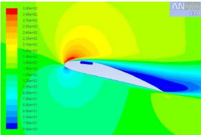
Fig. 9: Velocity variation on airfoil at 15° angle of attack
