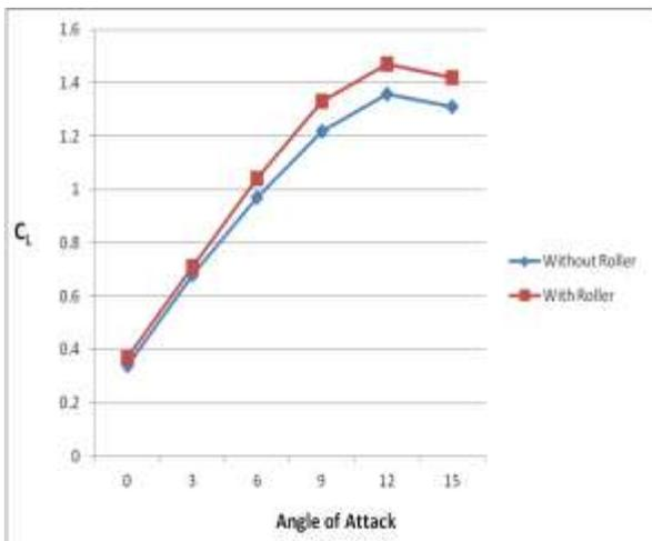
Fig. 18: Comparison of  $C_L$  for airfoils with and without roller at different AoA
