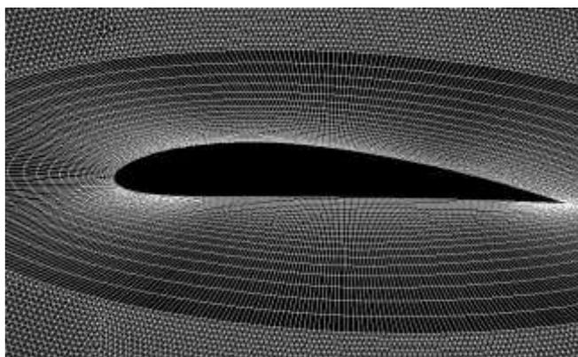
Fig. 2: 2-D Grid system of a NACA 4412 airfoil
