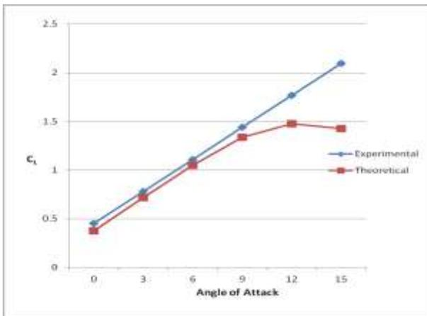
Fig. 17:  $C_L$  Vs Angle of attack
