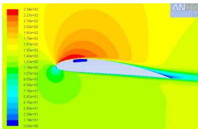
Fig. 7: Velocity variation on airfoil at 9° angle of attack
