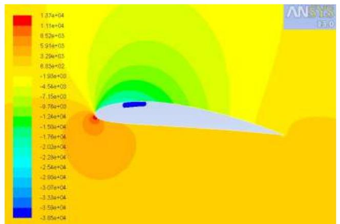
Fig. 13: Pressure variation on airfoil at 9° angle of attack
