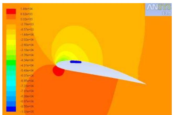
Fig. 14: Pressure variation on airfoil at 12° angle of attack
