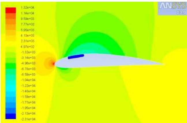
Fig. 10: Pressure variation on airfoil at 0° angle of attack
