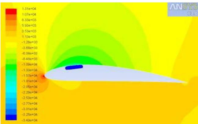
Fig. 11: Pressure variation on airfoil at 3° angle of attack
