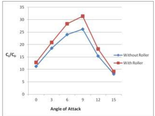
Fig. 19: Comparison of  $C_L/C_D$  for airfoils with and without roller at different AoA
