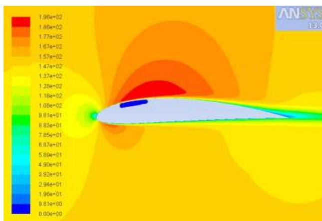
Fig. 4: Velocity variation on airfoil at 0° angle of attack
