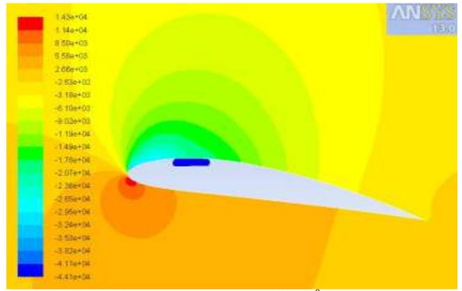
Fig. 12: Pressure variation on airfoil at 6° angle of attack
