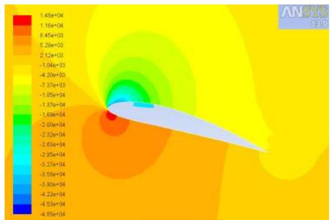
Fig. 15: Pressure variation on airfoil at 15° angle of attack
