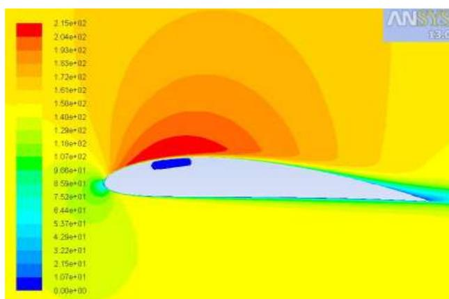
Fig. 5: Velocity variation on airfoil at 3° angle of attack
