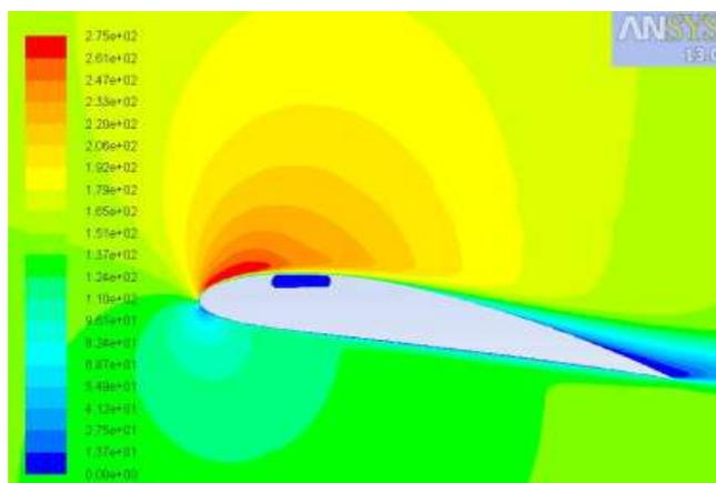
Fig. 6: Velocity variation on airfoil at 6° angle of attack
