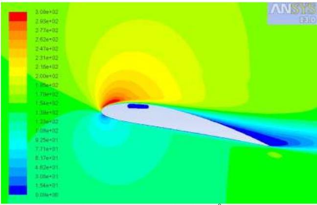
Fig. 8: Velocity variation on airfoil at 12° angle of attack
