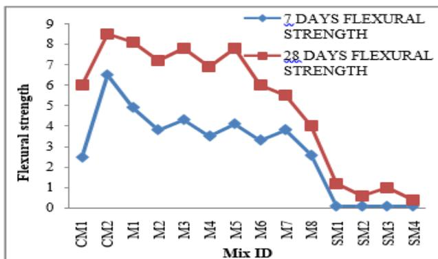
Fig. 8: 7 Days and 28 Days Flexural Strength Test Result of Control Mix And Partial Replacement of Cement with Fly Ash and GGBS Using 1% and 4% Sp.
