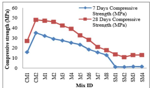
Fig. 6: 7 and 28 Days Compressive Strength Test Result of Control Mix And Partial Replacement of Cement with Fly Ash and GGBS Using 1% and 4% Sp.
