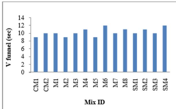
Fig. 3: V-Funnel Value of Control Mix and Partial Replacement of Cement with Fly Ash and GGBS Using 1% and 4% Sp.
