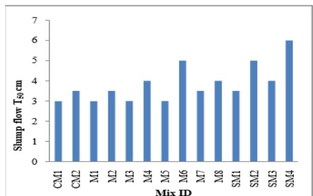
**Fig. 2:** Slump Flow T50 Cm Value of Control Mix and Partial Replacement of Cement with Fly Ash and GGBS Using 1% and 4% Sp.
