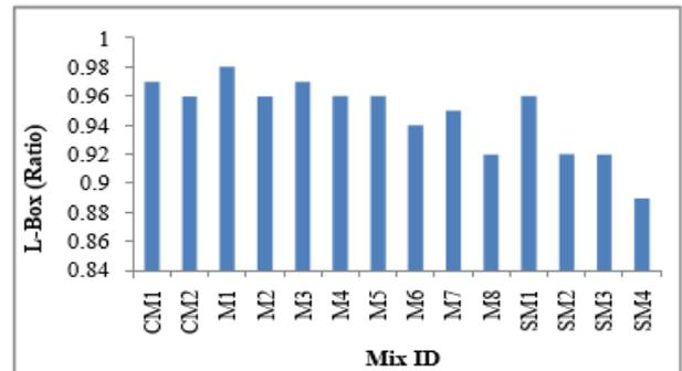
Fig. 5: L-Box of Control Mix and Partial Replacement of Cement with Fly Ash and GGBS Using 1% and 4% Sp.
