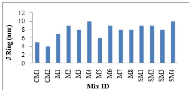
Fig. 4: J-Ring of Control Mix and Partial Replacement of Cement with Fly Ash and GGBS Using 1% and 4% Sp.
