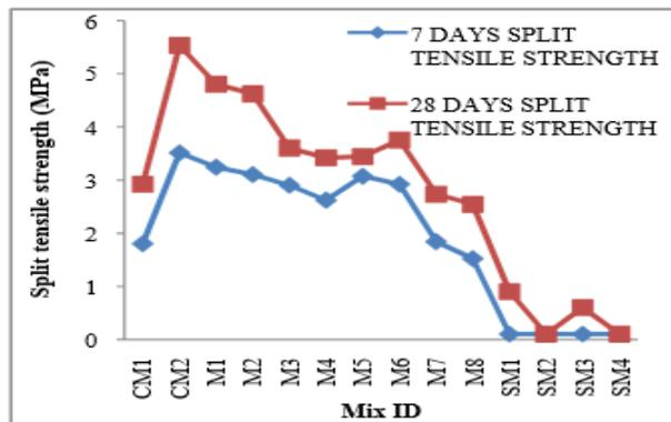
Fig. 7: 7 and 28 Days Split Tensile Strength Test Result of Control Mix and Partial Replacement of Cement with Fly Ash and Ggbs Using 1% and 4% Sp.
