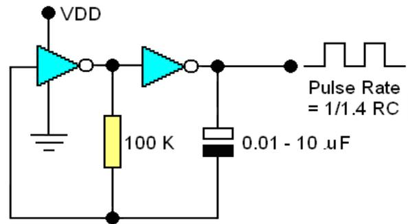
Fig. 4: Diagram of TTL Oscillator [5].
