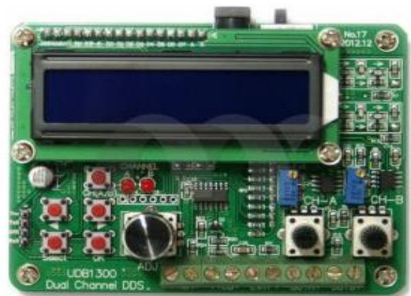
Fig. 5: Sample of Source Signal Generator [6].
