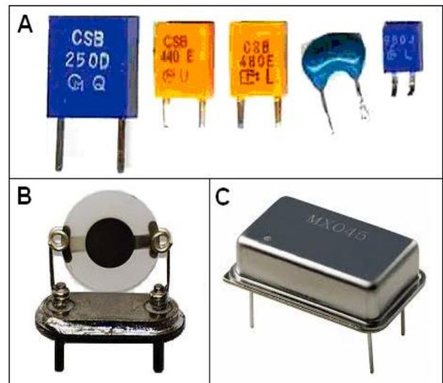
Fig. 12: Different Types of Resonators and Oscillators [9].
