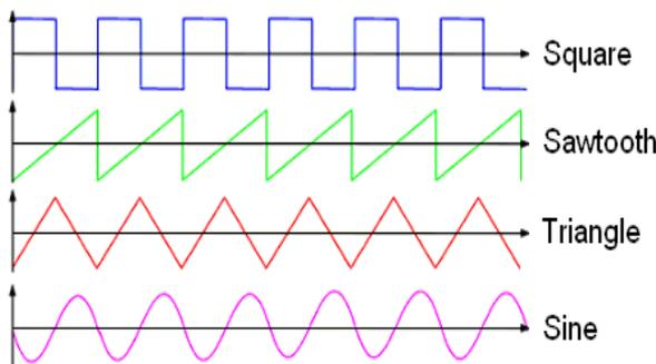
Fig. 3: AF Waveforms [4].
