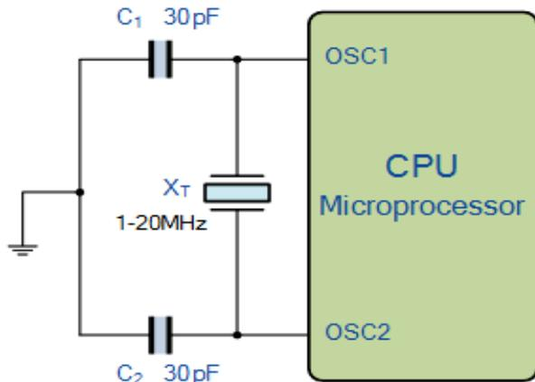
Fig. 10: Microprocessor Oscillator [7].
