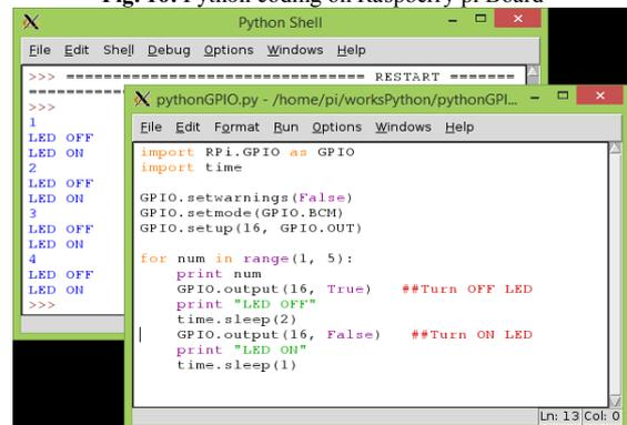
Fig. 17: GPIO LED Output
