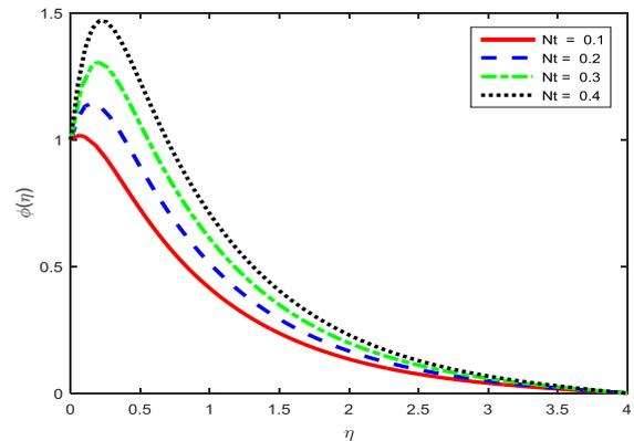
Fig. 6: Effect of thermophoresis parameter on concentration profiles
