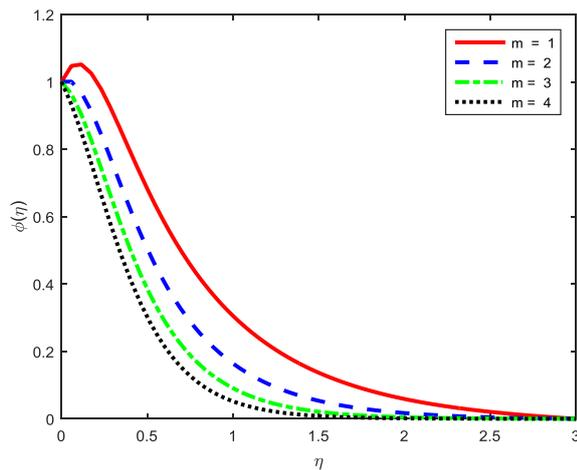
Fig. 8: Effect of Marangoni ratio parameter on concentration profiles
