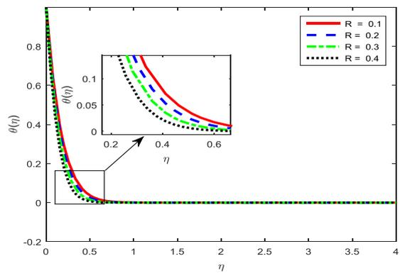
Fig. 2: Effect of Radiation parameter on temperature profiles
