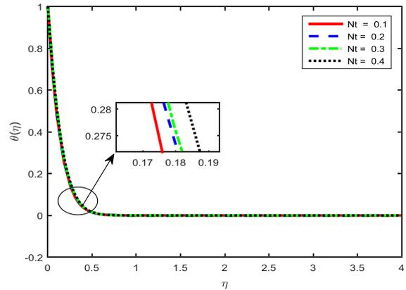
Fig. 5: Effect of thermophoresis parameter on temperature profiles
