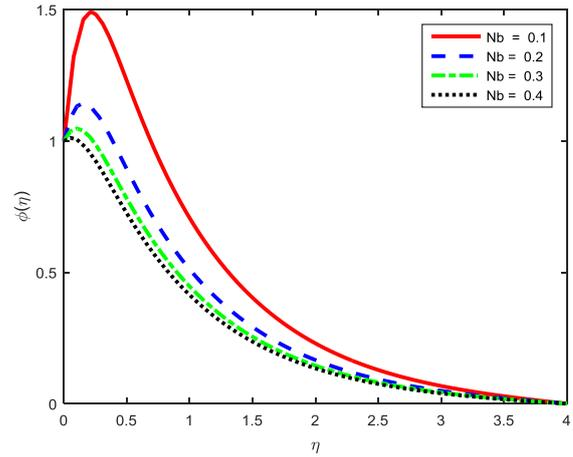
Fig. 4: Effect of Brownian motion parameter on concentration profiles
