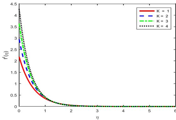
Fig. 1: Effect of porosity parameter on velocity profiles
