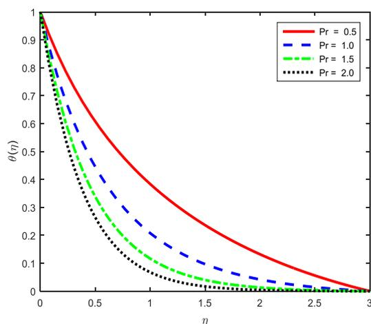
Fig. 10: Effect of Prandtl number parameter on temperature profiles
