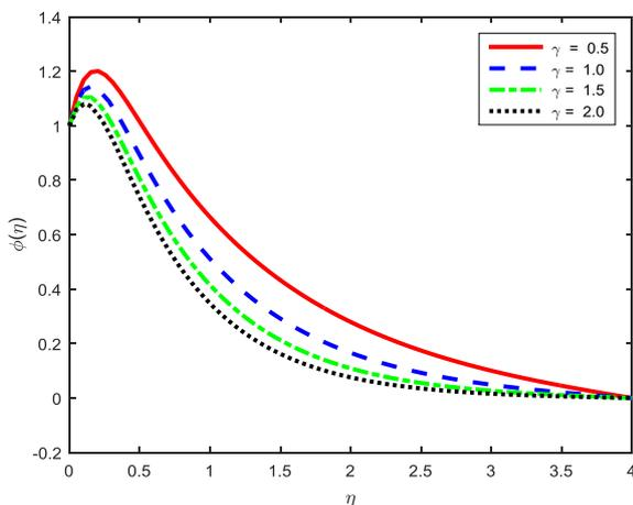
Fig. 3: Effect of chemical reaction parameter on concentration profiles
