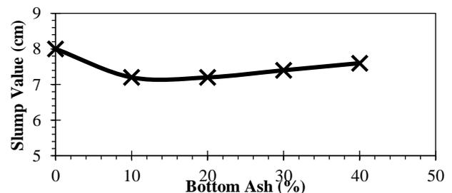
Fig. 1: The Slump Value of Concrete with Bottom Ash.
