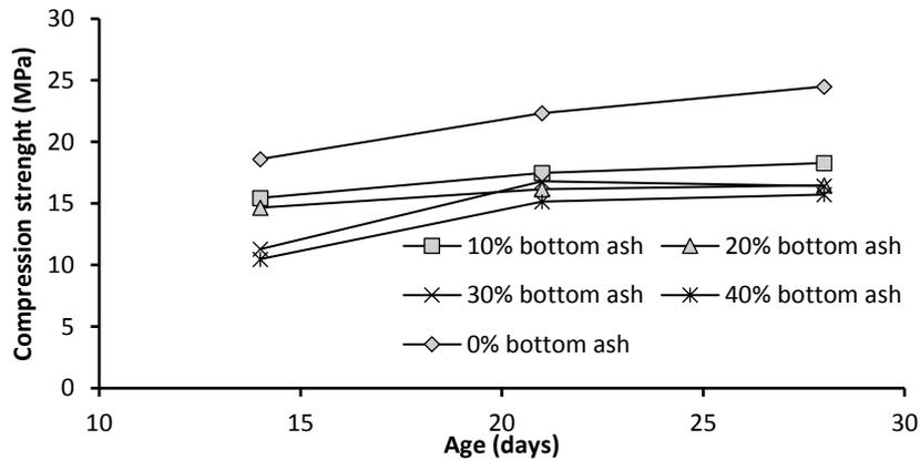
**Fig. 3:** Compression Strength Value of Concrete with Bottom Ash.
