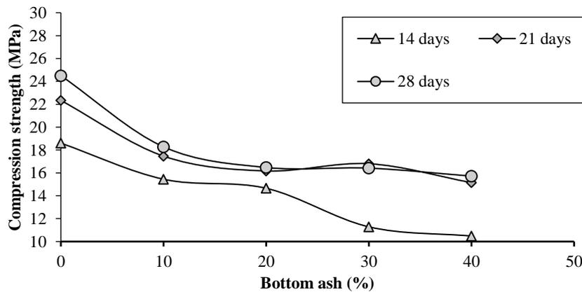
**Fig. 4:** Relationship of % Bottom Ash and Compression Strength.
