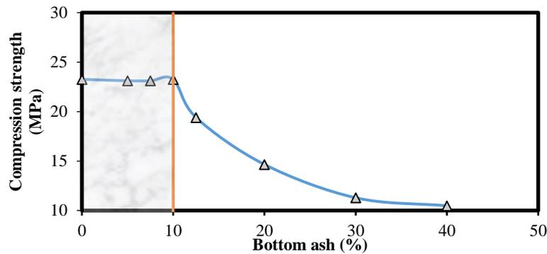
Fig. 5: Optimum Compression Strength of Concrete with Bottom Ash.
