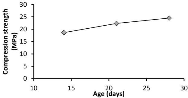
**Fig. 2:** Compression Strength Value of Concrete without Bottom Ash.
