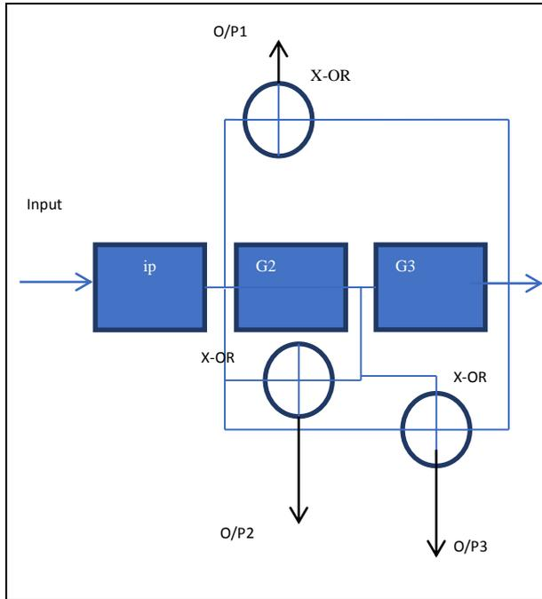
Fig. 4: The Structure of Convolution Coder.
