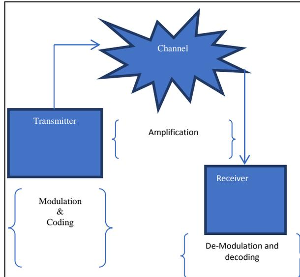
Fig. 1: Communication System Components.
