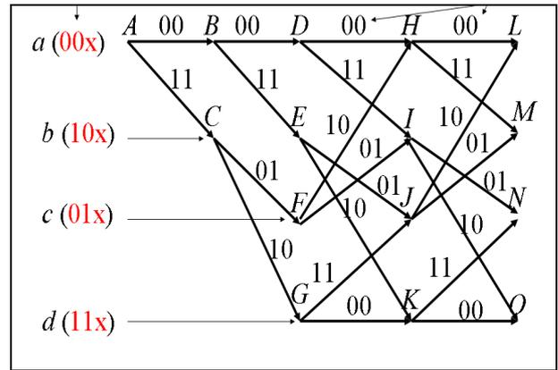
Fig. 5: Trellis Diagram That Obtain from Transition Table.
