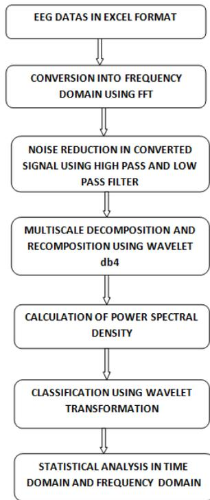
Fig. 2: Overall block diagram
