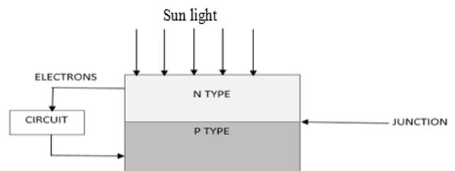
Fig. 1. Transection of Solar Cell
