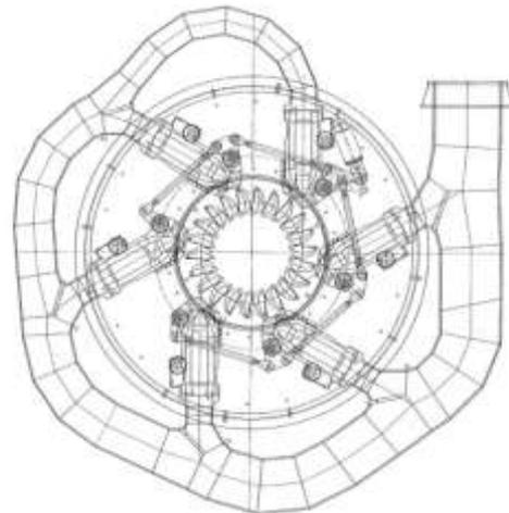
Fig. 1: Multi Nozzle distributor arrangement.
