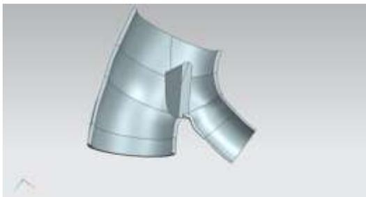
**Fig. 3:** wye branch of distributor (inner face)
