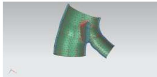
**Fig. 5:** Loading & Boundary Condition on wye branch
